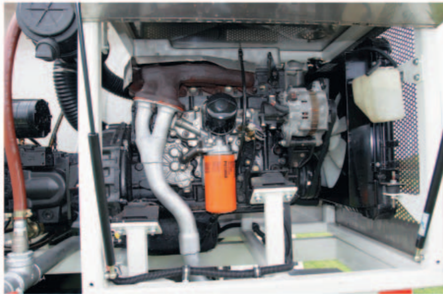
A Nissan FD42 provides the power needed to spread the viscous fluid down the high pressure hose.
