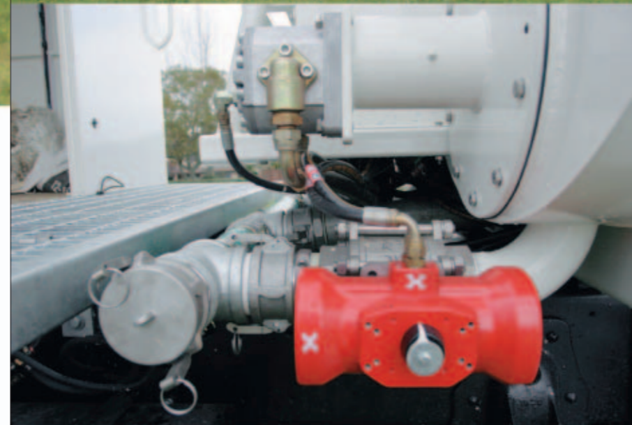
Valves controlling the flow of the fluid containing grass seed and fertiliser can be operated remotely from up to 150m away.
