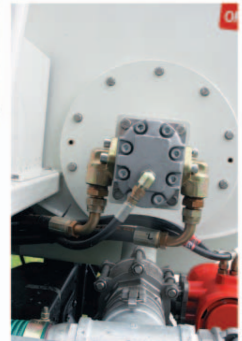
The mixing device is fitted to just the front end on both of the twin tanks.
