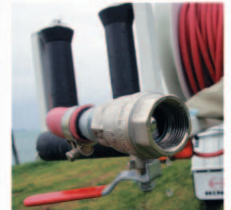
The high pressure delivery feeds through a boom keeping it free from tangling around the truck.
